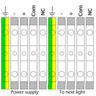
230V AC Com Com NC T N Ν ī. 0 0 0 0 0 0 0 To next light Power supply
